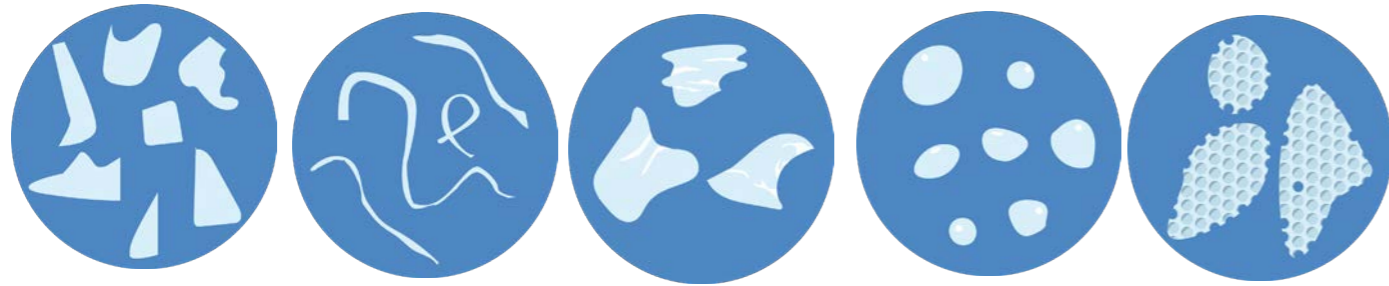
Figure 11: Common shapes of microplastics found in the marine environment: fragments, fibres, films, nurdles/pellets, foam.
