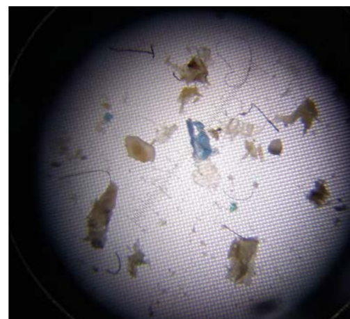
Figure 12: Microscope image of microplastic particles from seawater in the harbour of San Cristobal island. ©Jen Jones
